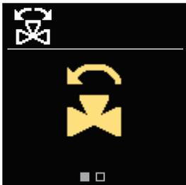
You can select the opening direction of the mixing valve. Use the buttons  $\ominus$  and  $\oplus$  to navigate between directions. Confirm the selected direction with the  $\odot$  button.
