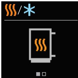
Use the buttons  $\ominus$  and  $\oplus$  to select the requested operating mode - heating or cooling.
