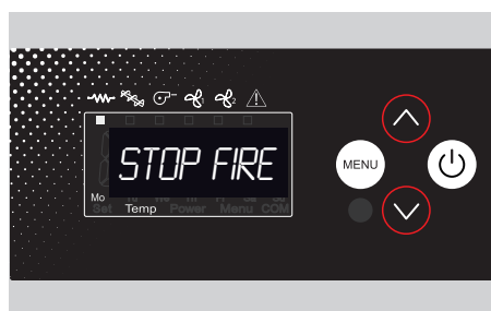
STOP FIRE The stove is in brazier cleaning. The fume extractor works at full speed.
