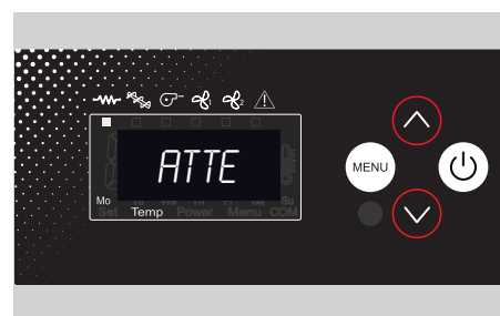
ATTE It appears when trying to restart the stove during the cooling cycle. Wait for the switching off cycle to complete, clean the brazier and proceed with a new ignition.
