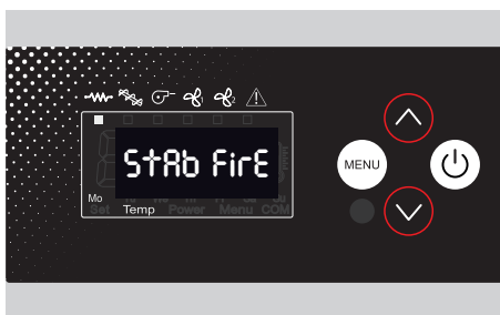
STAB FIRE The stove stabilizes after reaching the minimum ignition temperature. The electrical resistance turns off. The fume extractor and alternately the auger leds light up on the display.
