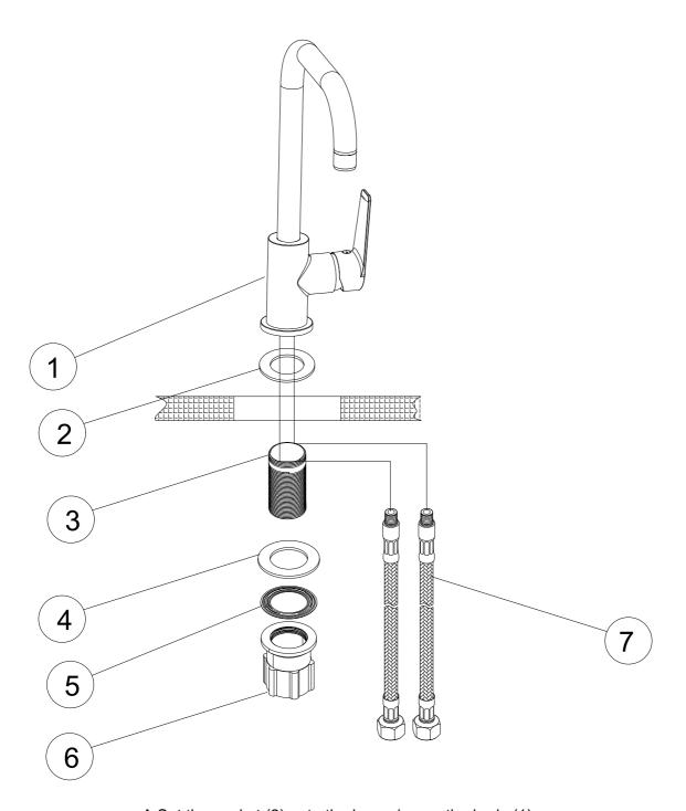
A.Set the gasket (2) onto the base ring on the body (1).
