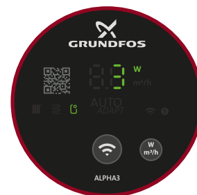
Fig. 32 Operating panel in "Automatic night setback"
