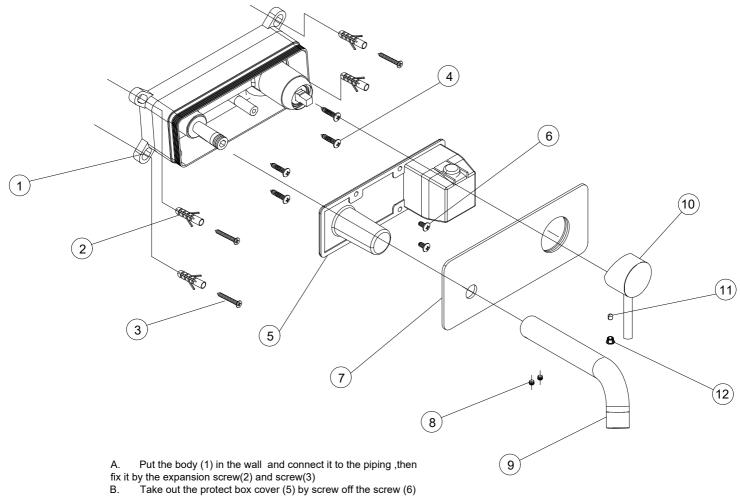
C. Put the panel (7) onto the body(1)
