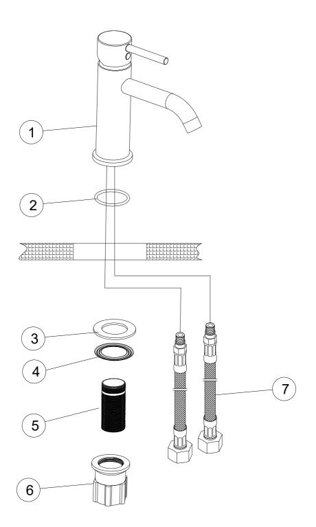
A.Set the o-ring (2) onto the base ring on the body (1).
