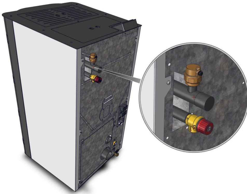
Picture 15. The representation of the air vent and safety valve at the back of the boiler
